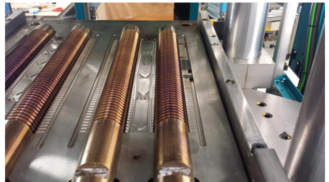
Figure 8 View of the 4-core mould for seals ND50
