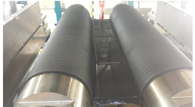
Figure 7 View of the seals ND110 on the core bars
